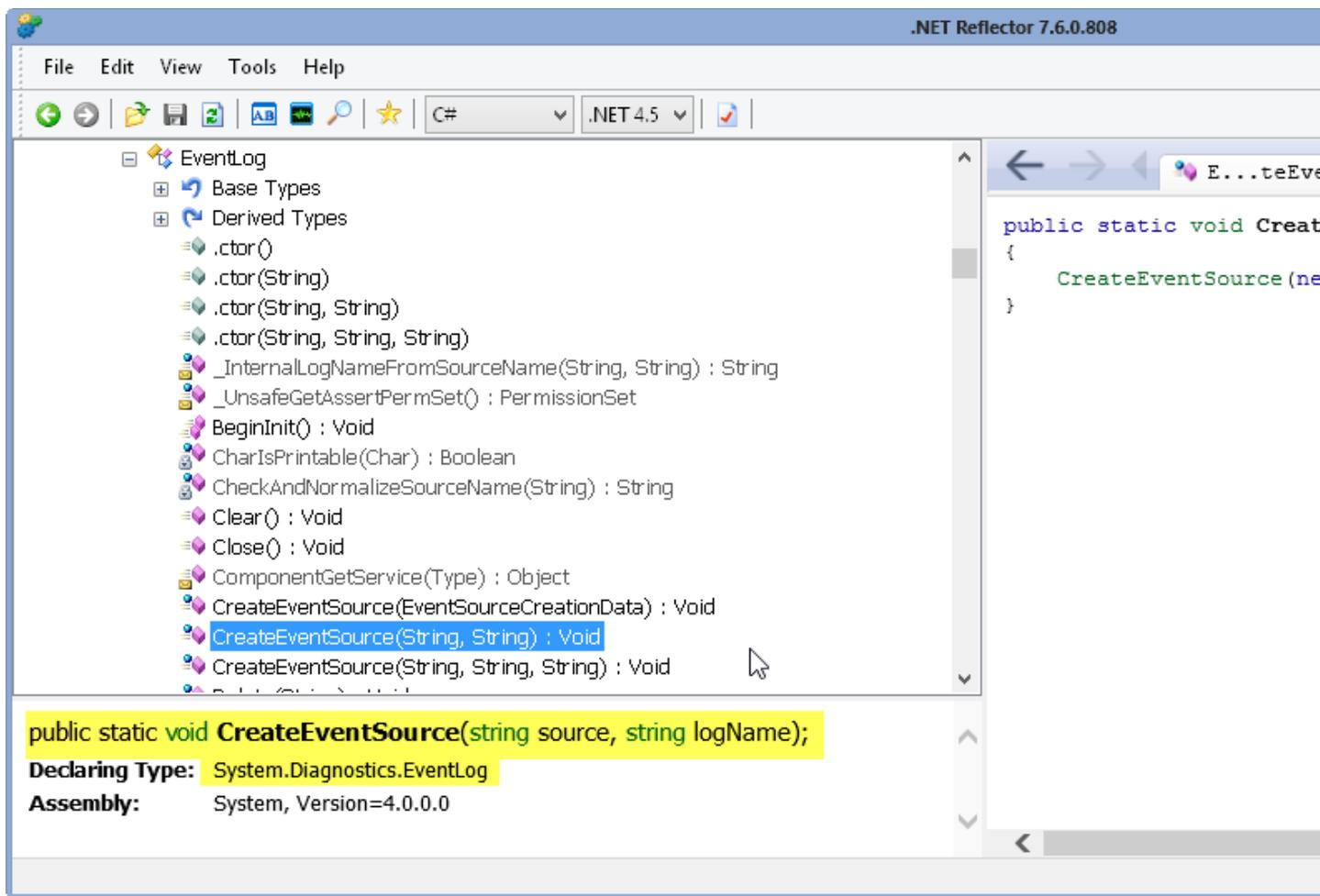
**Figure 7** – Reflector is a great tool to browse the .NET Framework libraries or any .NET assembly and see what functionality is available. Most code also is also viewable in decompiled mode, unless obfuscated explicitly.
