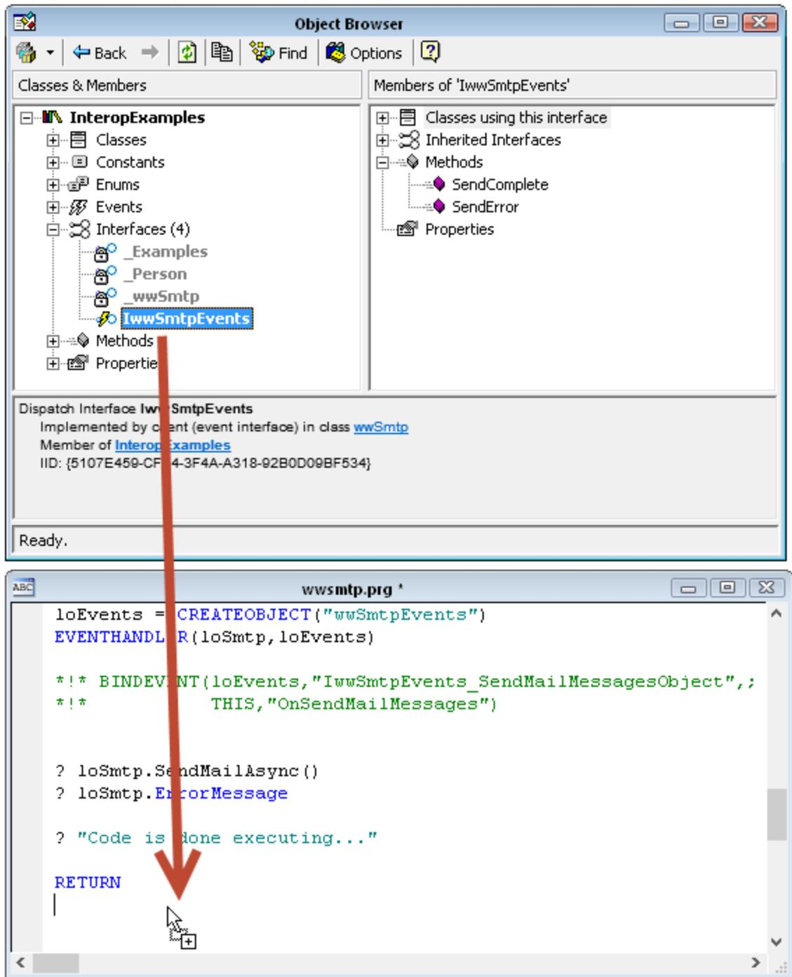
**Figure 9** – Dragging and dropping an Event Interface into a FoxPro PRG from the Object browser creates the COM event interface.
